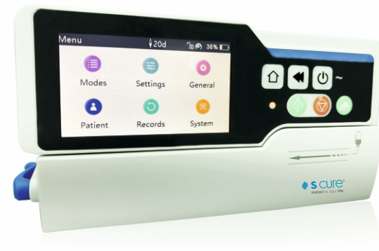
Touch Screen with 3 infusion modes & 4 Level of Occlusion
